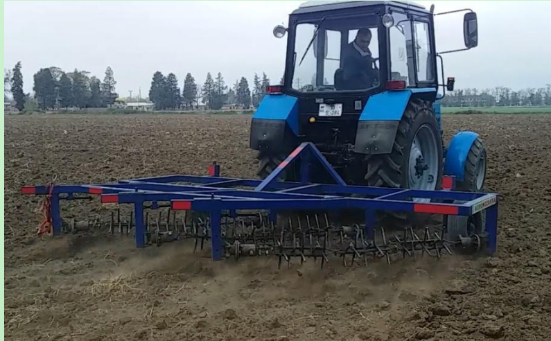
Figure 2. Field test of a flexible cable-driven rotary harrow
