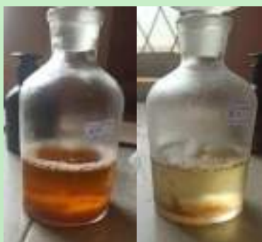
Figure 7. The supernatants were saturated with 80% ammonium sulfate for protein precipitation
