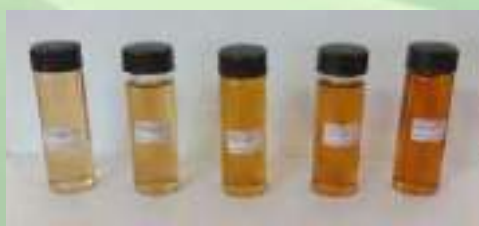
Figure 9. Serial Dilution of Methyl Orange for Absorbance/Indicator Studies
